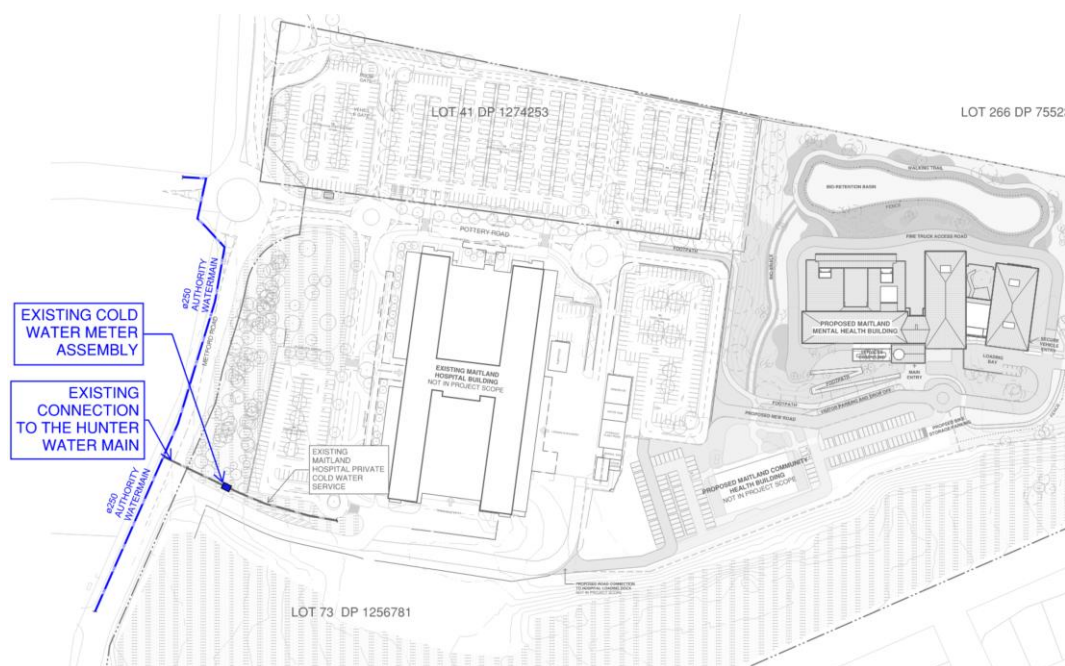
Figure 7 – Existing Connection to Authority Water Main
